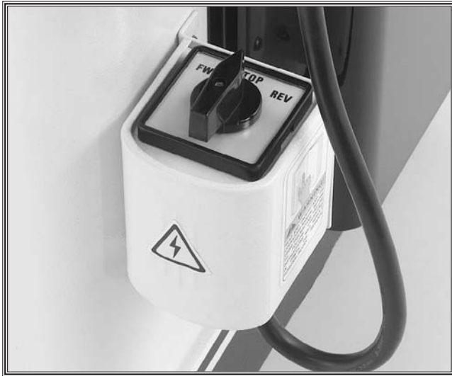
Figure 32. Forward and reverse switch.
