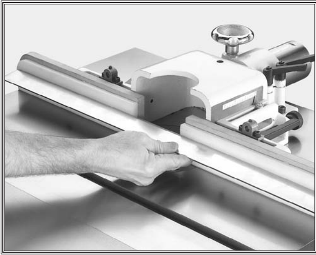
Figure 23. Use straightedge to check fence.
