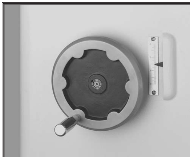
Figure 41. Spindle height handwheel.
