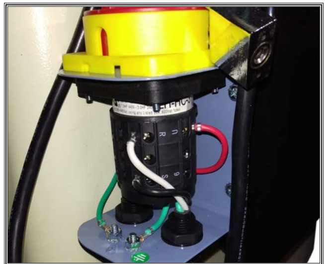
Figure 10. Forward/reverse switch wiring.
