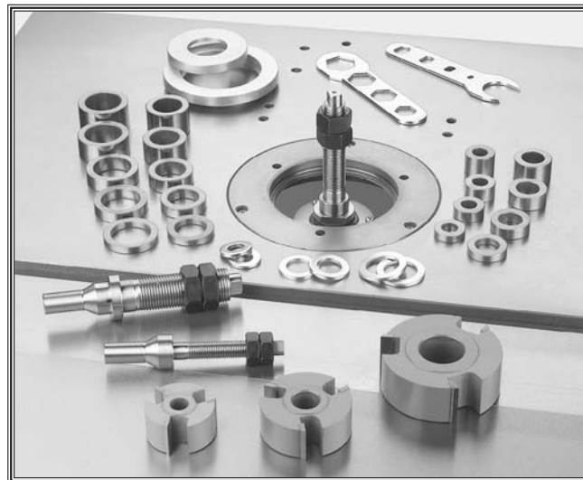
Figure 33. Common shaper hardware.
