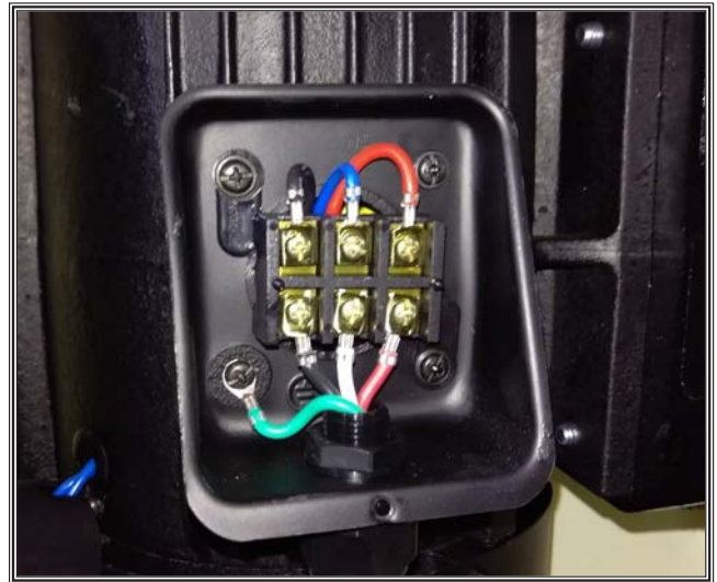
Figure 9. Updated motor wiring.
