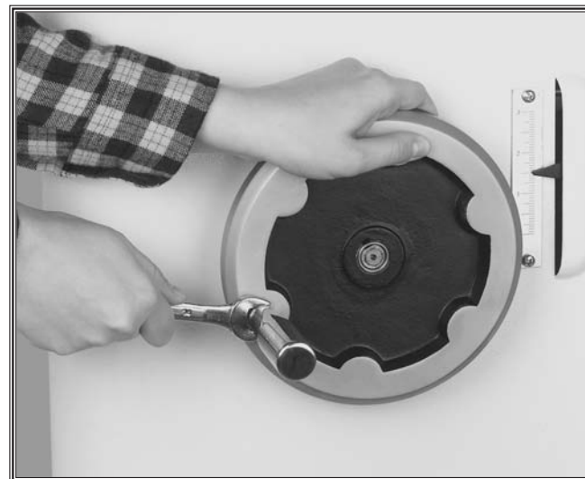
Figure 17. Attaching the crank handle.
