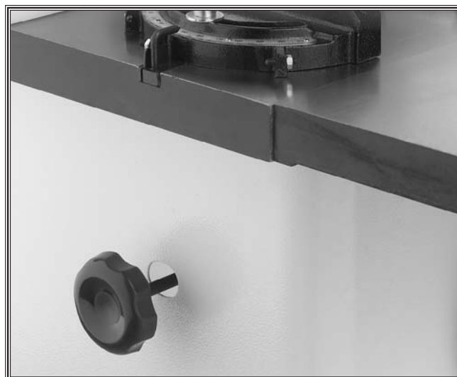
Figure 40. Spindle lock knob.
