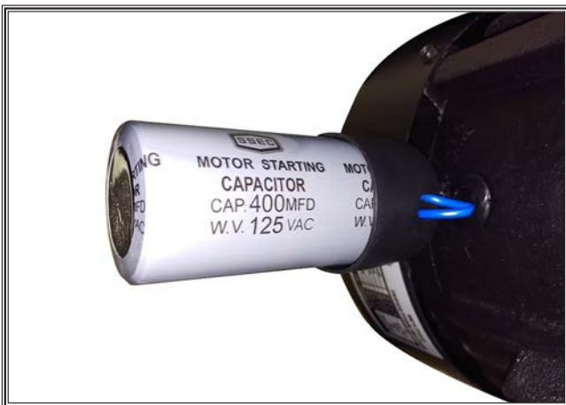
Figure 8. Updated motor start capacitor.
