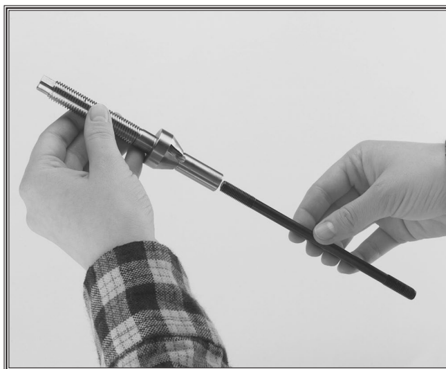
Figure 18. Threading drawbar into spindle.
