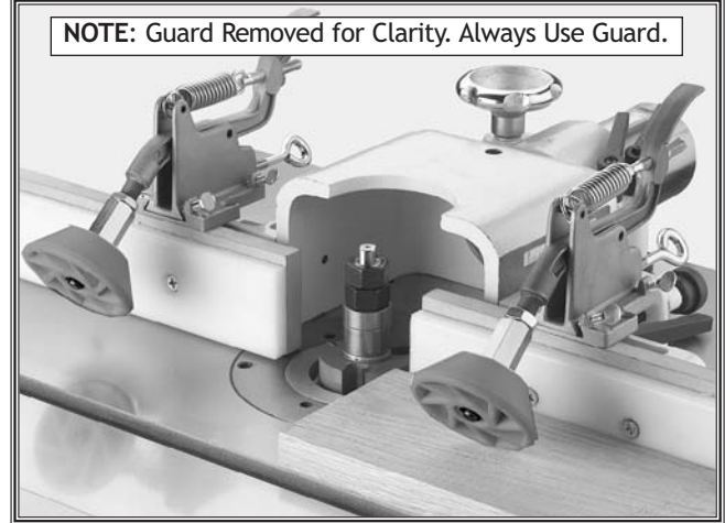
Figure 4. Use SHOP FOX® BOARD BUDDIES® for holding down the workpiece.
